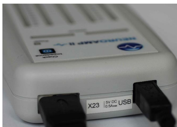
Figure 5a: USB connection between computer and EEG NeuroAmp II.5s and x23/x39-connection for accessories. Note: The x23-connection is available only for the model EEG NeuroAmp II.5s (A001001) device with a grey housing.
